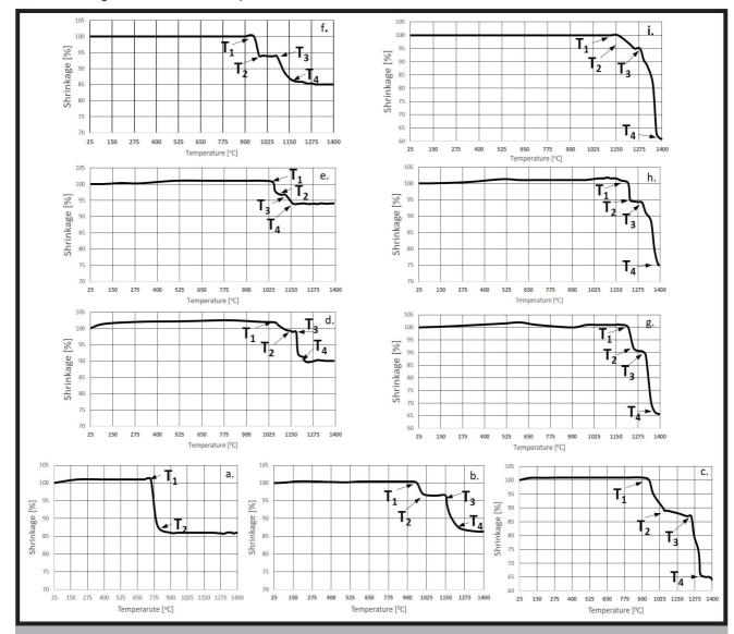
FIG. 2. Shrinkage curves derived from the HSM as a function of temperature for SBG-β-TCP composites and reference materials. Where: a. - S2, b. - β-TCP, c. - A2, d. - 25S2-β-TCP, e. - 50S2-β-TCP, f. - 75S2-β-TCP, g. - 25A2- β-TCP, h. - 50A2- β-TCP, i. - 75A2-β-TCP.
