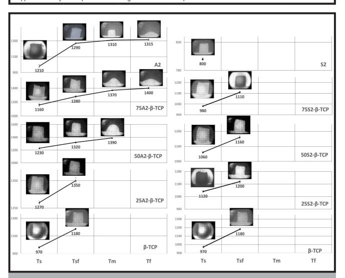
FIG. 3. The characteristic temperatures with correlated HTM images for A2-β-TCP, S2-β-TCP composites and reference sample ( $\beta$ -TCP, A2, S2). Where:  $T_s$  - initial shrinkage temperature,  $T_{sf}$  - softening temperature,  $T_m$  - melting temperature,  $T_f$  - flowing temperature.
