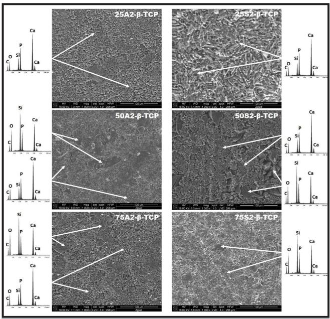
FIG. 4. SEM pictures and EDX spectra of SBG-βTCP composites.
